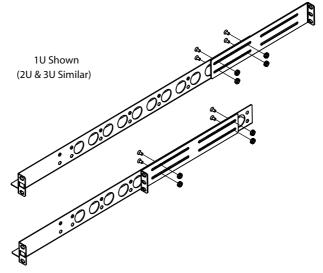
Step 2 Front Rack Attachment: Attach the front of each Fixed Rail to the rack using hardware from the Rack Hardware Kit (see Page 2).
