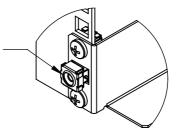
Step 1 Rail Assembly: Attach the Rear Brackets to each Fixed Rail using (4) 8-32 Flat Head Screws and (4) 8-32 Nuts. Always install the (4) screws and nuts as widely spaced as possible.
