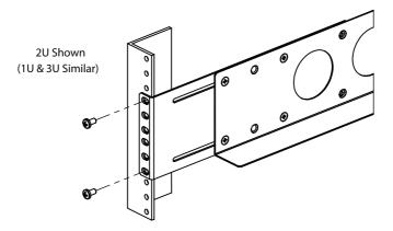
Step 4 <u>Cable Crossbar Attachment</u>: Attach the Cable Crossbar to the rack using hardware from the Rack Hardware Kit (see Page 2). The Cable Crossbar can be co-located with the Fixed Rails (as shown below). The Cable Crossbar can be installed in other locations as needed.
