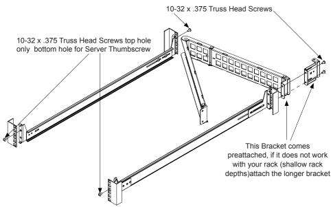
**Step 4.** <u>Mount Box:</u> Fully extend the rails first into their locked position, then slide the chassis in carefully using two people.
