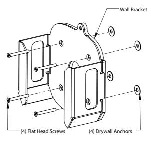
Step 5 <u>Install Dock:</u> Slide the docking station into the Wall Bracket. Consider cable management when placing your docking station.
