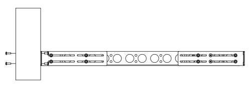
**Step 2b.** <u>Squared Rack Attachment:</u> Use Spacer with Pems if your application is using squared hole or 12-24 Racks. Spacers not required if using a 10-32 Rack.
