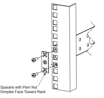
Note: 8-32 Hardware will feed thru 10-32 or 12-24 Racks into Fixed Rails.
