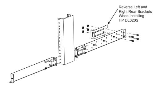
Step 2. Cable Crossbar Attachment: Attach the Cable Crossbar to the rack using hardware from the Assembly Hardware Kit (see Page 2).
