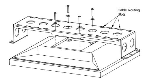
**Step 2.** Rack Mounting: Attach the Monitor and Mounting Bracket Assembly from Step 1 to the Rack, using (6) of the appropriate Rack Mounting hardware (see below).
