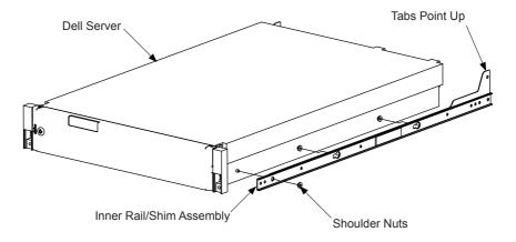
Step 3. Mount Outer Rail Assemblies: Mount both rails in the Rack as shown below.
