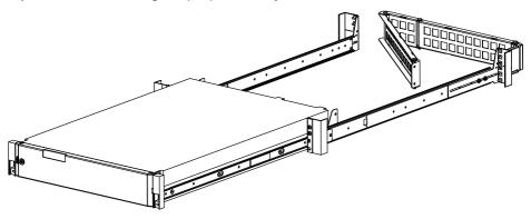
Step 3. Attach CMA: Attach the CMA Bracket to the inner shim, using the specified hardware.
