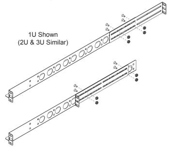
Step 2. <u>Front Rack Attachment:</u> Attach the front of each Fixed Rail to the rack using hardware from the Rack Hardware Kit (see Page 2).
