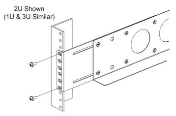
Step 4. <u>Cable Crossbar Attachment:</u> Attach the Cable Crossbar to the rack using hardware from the Rack Hardware Kit (see Page 2). The Cable Crossbar can be co-located with the Fixed Rails (as shown below). The Cable Crossbar can be installed in other locations as needed.
