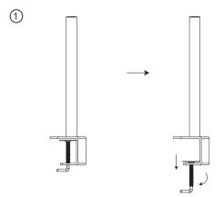
Loosen clamp screw until enough space is left for the edge of the desk.
