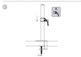
Adjust locating ring at proper height and screw up tight to hold the mount.
