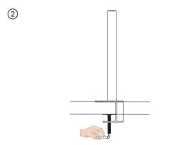
Tighten clamp using clamp screw until mount is securely fastened to desk.
