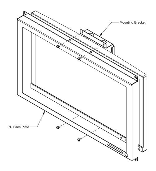
**Step 3** Rack Mounting: Attach the Monitor Mount to the Rack using (4) of the appropriate Rack Mounting hardware (see below).
