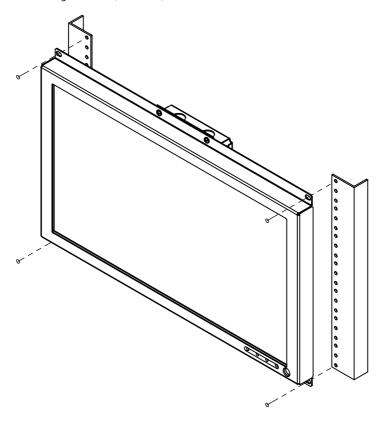
The Rack Hardware kit provides various screws and nuts for the four most common types of racks.
