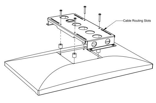
Step 2 Face Plate Attachment: Attach the Monitor Bracket Assembly to the 7U Face Plate as shown below using the supplied (4) 8-32 x .312 Pan Phil Screws.
