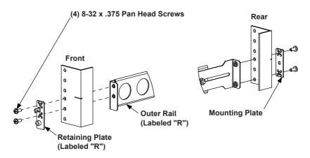
Step 4. Install the equipment: Slide the equipment all the way in. Tighten the (2)
