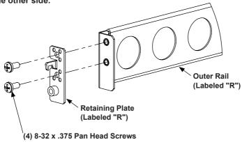
Step 5. Install the equipment: Slide the equipment all the way in. Tighten the (2)
