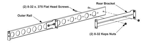
Step 3. Attach the rails to the rack: Attach the Front and Rear of the rails to the 4Post rack as shown below using supplied 8-32 Pan Head Screws on each side. Repeat for the other side. Right side shown, Left side parts are labeled "L". Tighten the front and rear Pan Head Screws on the right side rail. Leave the front and rear Pan Head Screws on the left side rail slightly loose.
