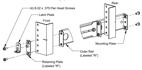
Step 4 Install the Equipment: Slide the equipment all the way in. Tighten the (2) Pan Head Screws on the back of the left slide rail. Slide the equipment out about 8 inches and tighten the (2) Pan Head Screws on the front of the left slide rail.
