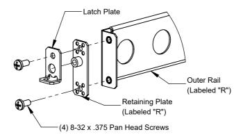
Step 5 Install the Equipment: Slide the equipment all the way in. Tighten the (2) Pan Head Screws on the back of the left side rail. Slide the equipment out about 8 inches and tighten the (2) Pan Head Screws on the front of the left slide rail.
