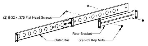
Step 3 Attach the rails to the rack: Attach the Front and Rear of the rails to the 2Post rack as shown below using supplied 12-24 Pan Head Screws on each side. Repeat for the other side. Right side shown, Left side parts are labeled "L". Tighten the front and rear Pan Head Screws on the right side rail. Leave the front and rear Pan Head Screws on the left side rail slightly loose.
