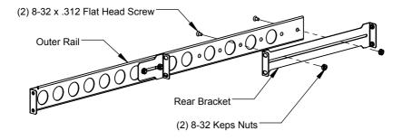
Step 3 Attach the Rails to the Rack: Attach the Front and Rear of the rails to the 4Post rack as shown below using supplied 8-32 Pan Head Screws on each side. Repeat for the other side. Right side shown, Left side parts are labeled "L". Tighten the front and rear Pan Head Screws on the right side rail. Leave the front and rear Pan Head Screws on the left side rail slightly loose.
