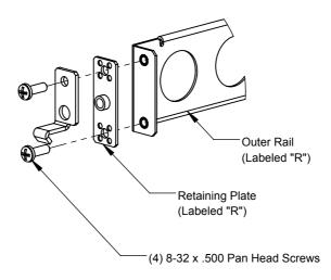
Step 5 Install the Equipment: Slide the equipment all the way in. Tighten the (2) Pan Head Screws on the back of the left side rail. Slide the equipment out about 8 inches and tighten the (2) Pan Head Screws on the front of the left slide rail.
