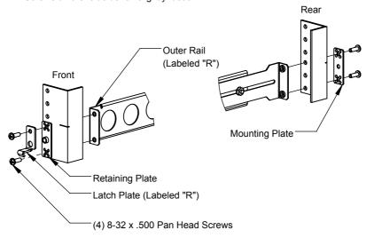
Step 4 Install the Equipment: Slide the equipment all the way in. Tighten the (2) Pan Head Screws on the back of the left slide rail. Slide the equipment out about 8 inches and tighten the (2) Pan Head Screws on the front of the left slide rail.
