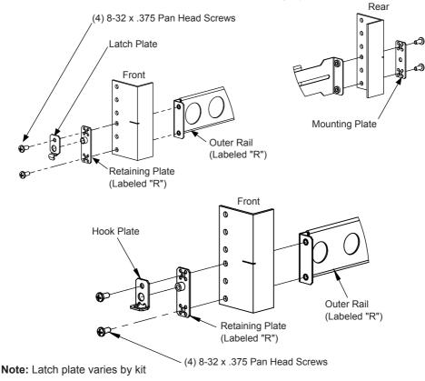
**Step 4.** <u>Install the equipment:</u> Slide the equipment all the way in. Tighten the (2) Pan Head Screws on the back of the left slide rail. Slide the equipment out about 8 inches and tighten the (2) Pan Head Screws on the front of the left slide rail.
