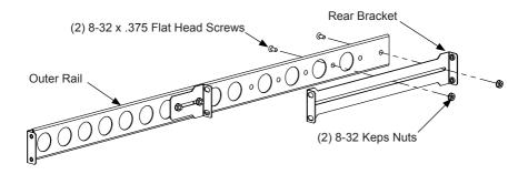
Step 3. Attach the rails to the rack: Attach the Front and Rear of the rails to the 4Post rack as shown below using supplied 12-24 Pan Head Screws on each side. Repeat for the other side. Right side shown, Left side parts are labeled "L". Tighten the front and rear Pan Head Screws on the right side rail. Leave the front and rear Pan Head Screws on the left side rail slightly loose.
