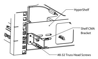
Remove Screw: Remove the (1) Truss Head Screw that is located at the left rear of Step 4 the rack.
