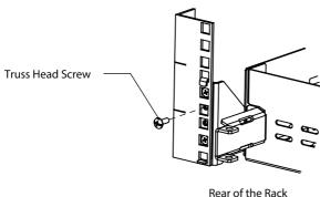
Step 5 Secure the Cable Managment Arm: Secure the Cable Managment Arm to the rack by installing (1) 8-32 x .500 Truss Head Screw provided in the Cable Managment Arm Kit and the screw from the previous step through the Rack Mounted Cable Managment Bracket.
