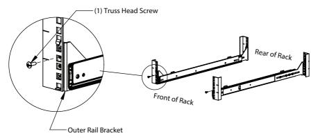
Step 1b Secure Rail Assemblies: Secure the rear of the rail assemblies by installing (1) 8-32 x .500 Truss Head Screw into the right and left Outer Rail Bracket.
