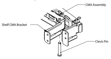
Step 3b Mount Shelf CMA Bracket : Secure the Shelf CMA Bracket to the rear (left side) of the HyperShelf using the provided (2) #8-32 Truss Head Screws
