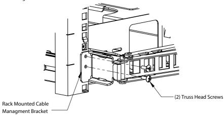
Step 6 Fasten Shelf CMA Bracket: Re-attach the Clevis Pin that fastenes the Shelf CMA Bracket to the CMA Assembly using the paired Cotter Pin.
