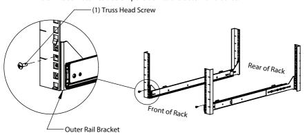
Step 1b Secure Rail Assemblies: Secure the rear of the rail assemblies by installing (1) 8-32 x .500 Truss Head Screw into the right and left Outer Rail Bracket.
