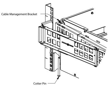
Step 3b Secure the Cable Managment Arm: Secure the Cable Managment Arm to the rack by installing (2) 10-32 x .500 Pan Head Screw provided in the Cable Managment Arm
