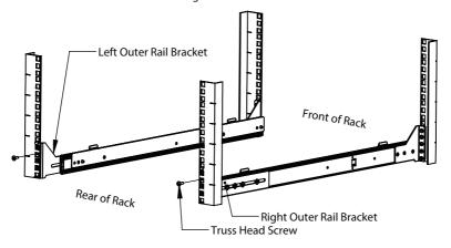
Step 2 <u>Install the HyperShelf:</u> With the rails fully extended and side panels removed, Align the shelf with the rail side tabs and place the shelf on the rails.
