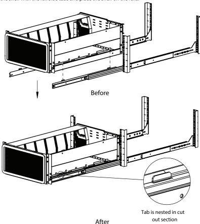
Step 2b Secure the HyperShelf: Secure the HyperShelf by installing (2) 8-32 x .250 Truss
