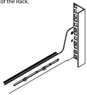
Step 1b Front Rack Attachment: Disengage the Latch and insert the Front Hook into the Square Holes of the Rack. Release the Latch which will return to the engaged position securing the Front of Rail. See detail view for Latch
