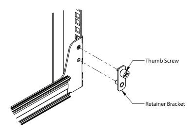
Step 3 Shelf Installation: Ensure the Rails are fully closed and the Retainer Brackets are properly installed on both sides. Ensure the Shelf is right side up. Align the Rail Tracts on the Shelf with the Rail Tracts on the Rack and insert the Shelf until the Safety Latch engages. Disengage the Release Latch on the front of the Rails and push the Shelf fully into the Rack. The Shelf can now be secured with the Thumbscrews.
