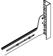
Step 1b <u>Front Rack Attachment:</u> Disengage the Latch and insert the Front Hook into the Square Holes of the Rack. Release the Latch which will return to the engaged position securing the Front of Rail. See detail view for Latch operation.
