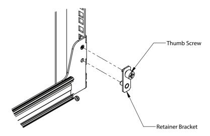
Step 3Shelf Installation:Ensure the Rails are fully closed and the Retainer<br/>Brackets are properly installed on both sides. Ensure the Shelf is right side<br/>up. Align the Rail Tracts on the Shelf with the Rail Tracts on the Rack and<br/>insert the Shelf until the Safety Latch engages. Disengage the Release<br/>Latch on the front of the Rails and push the Shelf fully into the Rack. The<br/>Shelf can now be secured with the Thumbscrews.
