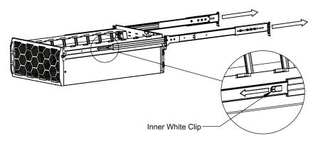
Step 2a Attach Outer Rails: Attach the outer rails to the rack by hooking the top of the Outer Rail Bracket into the top hole of the "U" space. Secure the rails by installing (1) Truss Head Screw per side into the Outer Rail Brackets.
