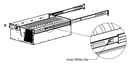
Step 2a Attach Outer Rails: Attach the outer rails to the rack by hooking the top of the Outer Rail Bracket into the top of the "U" space. Secure the rails by installing (1) Truss Head Screw per side into the Outer Rail Bracket.
