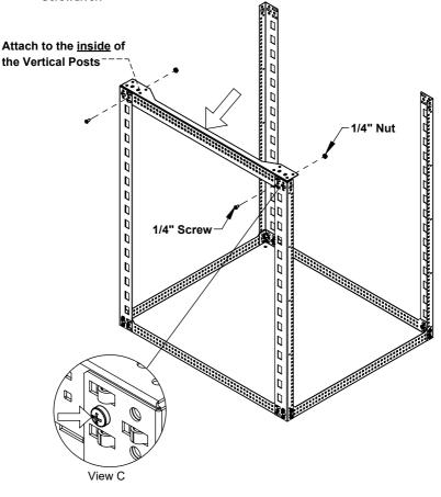
**Note:** During this step, attach Depth Bracket to each Vertical Post using only the 1/4" Screw shown in View C above.
