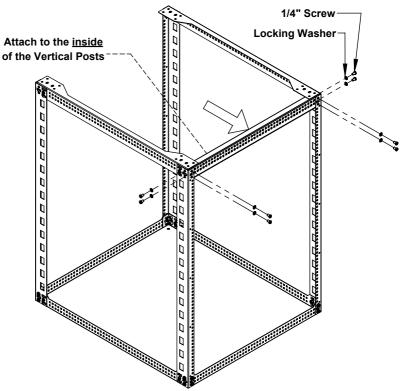
**Note:** When attaching Width Bracket, the (4) holes should be facing up, as shown in the picture below.
