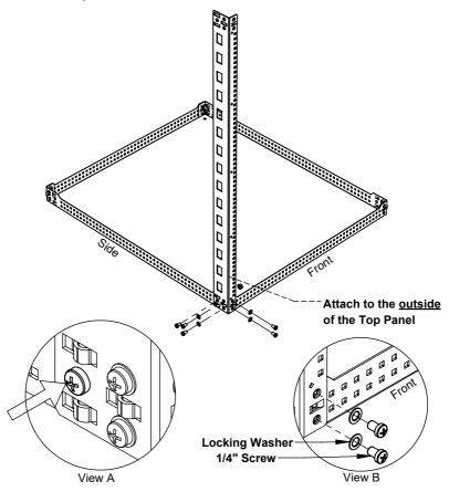
Note: To secure 1/4" Screw shown in View A above, place 1/4" Screw through hole in Vertical Post and Top Panel, and hand tighten 1/4" Nut onto Screw before using Screwdriver.
