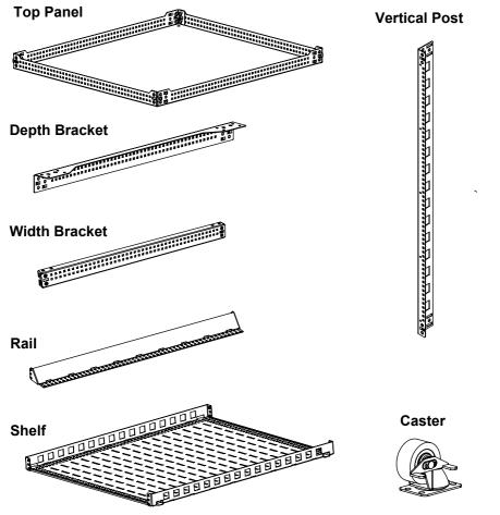
Step 1 Attach Vertical Post: Attach Vertical Post to <u>outside</u> of Top Panel using (5) 1/4" Screws, (4) Locking Washers, and (1) 1/4" Nut. Install the front (2) 1/4" Screws first, tighten each screw with Screwdriver, then install side (3) 1/4" Screws and tighten each with Screwdriver.
