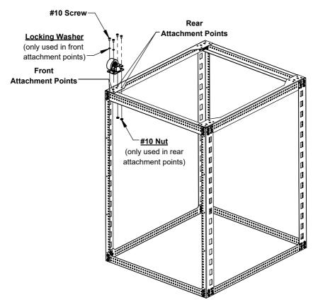
Note: When securing the (2) #10 Screws located in the Rear Attachment location, Place #10 Screw through hole in Caster and Depth Bracket, and hand tighten #10 Nut onto Screw before tightening with Screwdriver.
