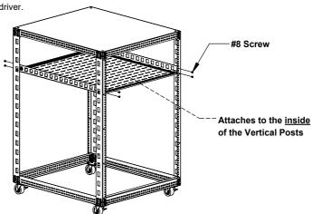
Step 7 Attach Rails: Attach Rails to the inside of the Vertical Posts using (4) #8 Screws per rail. Tighten each using Screwdriver.
