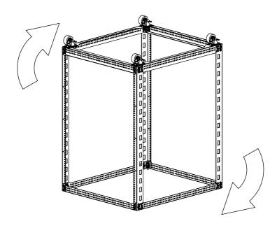
Step 6 Install Shelf: Install Shelf by rotating shelf into position. Insert Shelf Tabs into Vertical Post Cutout, and rotate the opposite side of the shelf, until Shelf is level. The opposite side Shelf Tabs should fit into opposite side Vertical Post Cutout.
