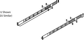
Front Rack Attachment: Attach the front of each Fixed Rail to the rack using Step 2 (2) 8-32 Pan Head Screws and (1) Square-hole Retainer Plate. Repeat for the other side.
