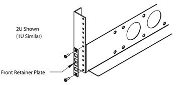
Note: Front and Rear Retainer Plates are different.
