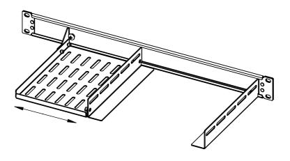
Step 3 Install Device and Lock Shelf in Position: Place the device on the shelf and tighten the #10-32 Screw to lock the shelf into place.
