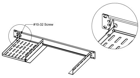
Step 2 Adjust Shelf Position: Slide the shelf to an appropriate width for mounting the device.
