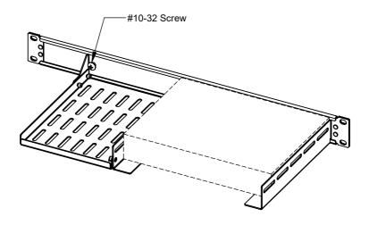
**Step 4** <u>Install Push-In Bumpers:</u> Slide the Push-In Bumpers to an appropriate location along the rear slots to secure the back of the device.
