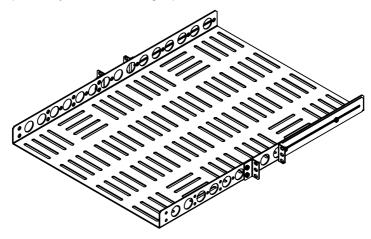
Step 3 Attach Shelf Assembly: Attach the shelf assembly to the rack as shown below using the Rack Hardware Kit. See Page 8 for rack hardware requirements.
