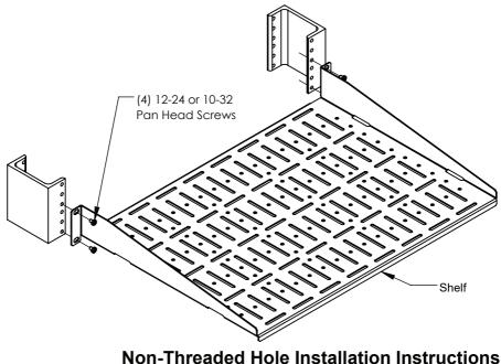
**Step 1** Line up shelf in desired U space and orientation. Attach with the following hardware.
