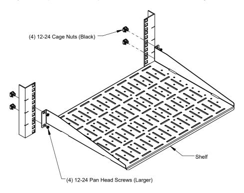
**Step 1** Line up shelf in desired U space and orientation. Attach with the following hardware.
