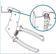
3. Tilt cage nut so the other prong is inside of the square hole
