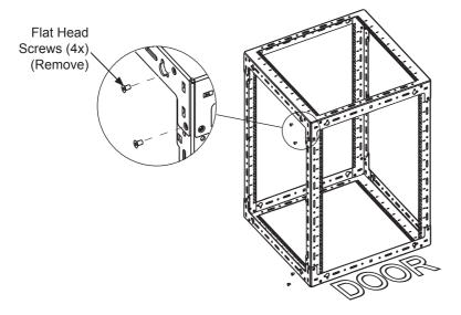
Step 2. <u>Attach Door Bracket:</u> Attach Door Bracket onto Rack using the Screws removed in Step 1. Install the additional Flat Head Screws, securing it with the Nylock Nuts on the opposite.
