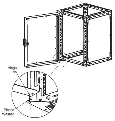
**Step 7**. <u>Install Door:</u> Align top hole and top pin hinge and install using included 10-32 flat head screws.
