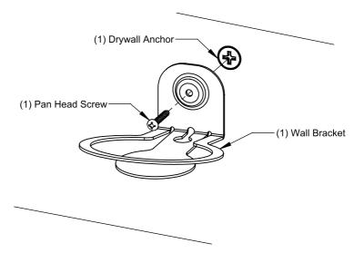
Note: Tighten until mount is secure to the wall. Do NOT overtighten screw.
