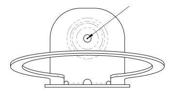
Step 3 Install Drywall Anchor: Install (1) Drywall Anchor at the marked hole. Using a #2 Philips head screwdriver, press the anchor into the drywall while turning clockwise until it is seated flush with the wall.
