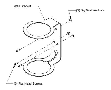
Step 5 Install the Wall Bracket: Place the cord through the bottom hole in the mount. Slide the Homepod into the mount, letting the cord fall through the back slot.
