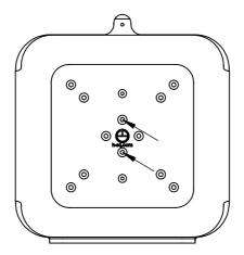
Step 3 Install Drywall Anchor: Install one Drywall Anchor at each hole mark. Using a #2 Phillips head screwdriver, press the anchor into the drywall while turning clockwise until it is seated flush with the wall.
