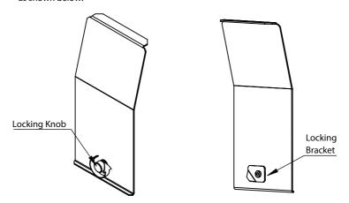
Step 2 Insert Blanking Panel: Insert the Blanking Panel into the desired slot location on the Hypershelf.
