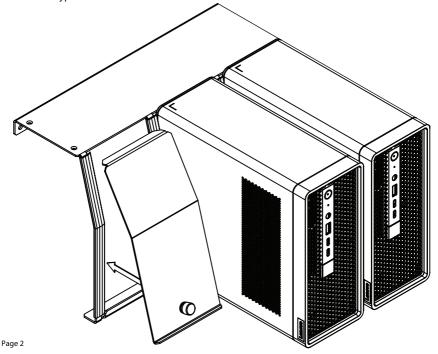
Step 3 Secure the Blanking Panel: Secure the Blanking Panel into place by turning the Locking Knob clockwise.
