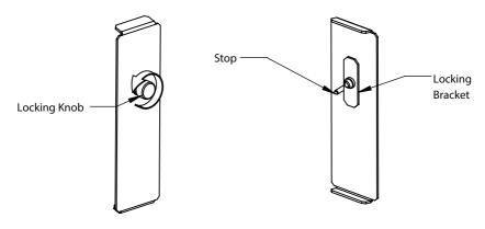
Step 2 <u>Insert Blanking Panel:</u> Insert the Blanking Panel into the desired slot location on the Hypershelf.
