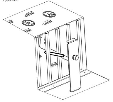
Step 3 <u>Secure the Blanking Panel:</u> Secure the Blanking Panel into place by turning the Locking Knob clockwise.
