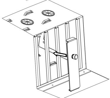
Step 3 Secure the Blanking Panel: Secure the Mac Mini Blanking Panel into place by turning the Locking Knob clockwise.
