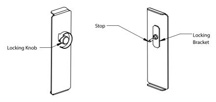
Step 2 Insert Blanking Panel: Insert the Mac Mini Blanking Panel into the desired slot location on the Hypershelf.
