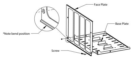
Step 2 <u>Attach Side Brackets:</u> Attach the two Side Support Brackets as shown below using (4) of the provided #8 screws.
