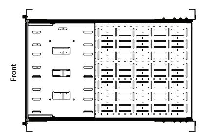
Step 4 Fasten the Bracket Set: Fasten the Bracket Set to the Modular Shelf with the (4) included nuts, as shown below.
