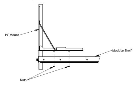
Step 5 Mount Devices to the Bracket Set: Slide the devices in between the gaps on the bracket set. Ensure the feet of each device are set into their placement cut-outs.
