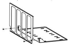
Step 2 Install brackets along the slot pattern of the shelf. Its recommended to mount the bracket in the frontmost postion on the shelf.
