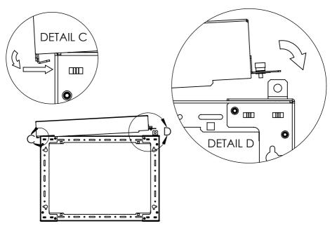
Step 4 <u>Lock Door:</u> Hook padlock (not included) through the hole on the locking bracket.
