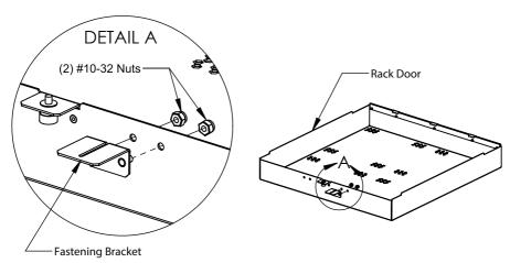
Step 2 <u>Attach Door Latch Bracket:</u> Secure Door Latch Bracket to rack with (2) #10-32 Nuts.
