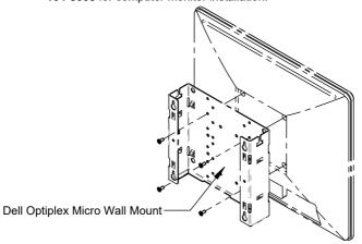
Step 2 Carefully insert the Dual VESA mounting bracket from the bottom of the Dell Optiplex Micro Wall Mount and secure with the #8 screws.
