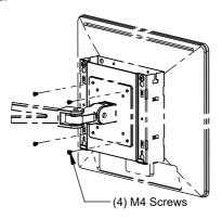
**Step 4** Carefully insert the computer into the Dell Optiplex Micro Mount.
