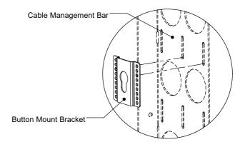
Step 2 Securing the Button Mount Bracket: Install the Pan Head Screws into the appropriate hole location and secure it to the Cable Management Bar with Kep Nuts.
